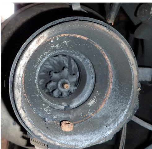
**Figure 19:** Mechanical failure of the turbo charger resulted in a failed oil seal.
