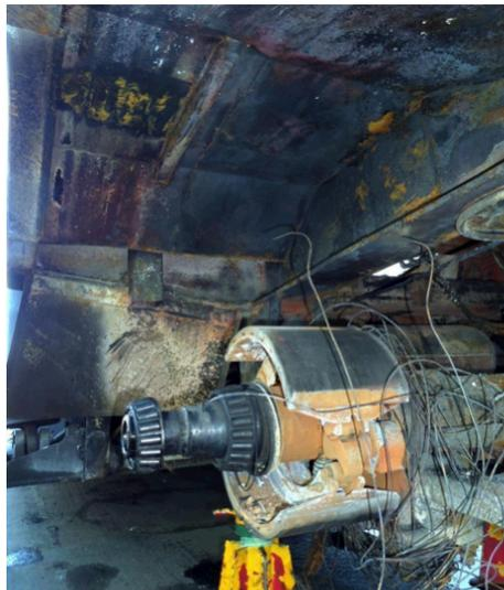
**Figure 25:** Fire caused by a tyre rub on a metal mudguard. Note the bearings have not failed.
