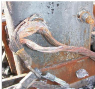
**Figure 11:** Re-routing of main battery cable to starter motor.
