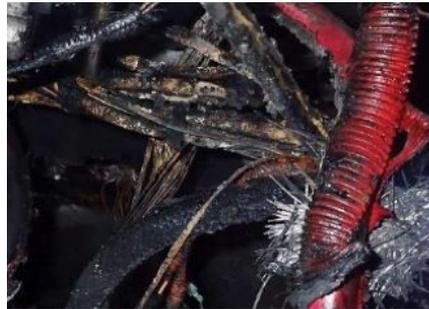
**Figure 10** Starter current flowed via the chassis-rail earth link, which overheated.
