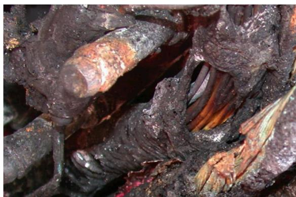
**Figure 5:** A fire the result of a rub between the alternator cable and an engine stud.
