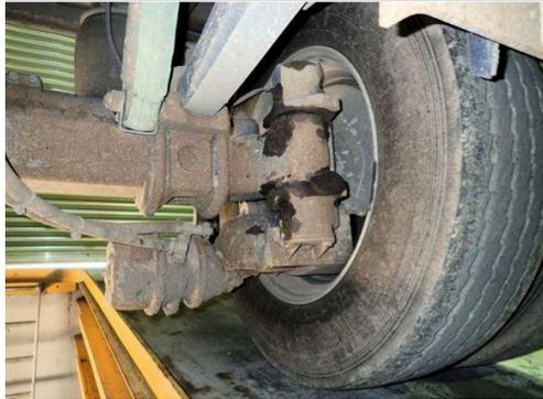
**Figure 21:** Low slung disc brake actuator.
