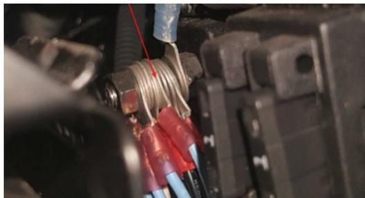
**Figures 14:** Stacking of ring terminals on a return stud in an aftermarket telemetry system.
