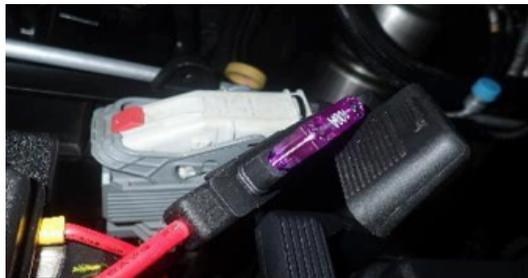
**Figures 13:** A 100A fuse in a 60A rated fuse holder.
