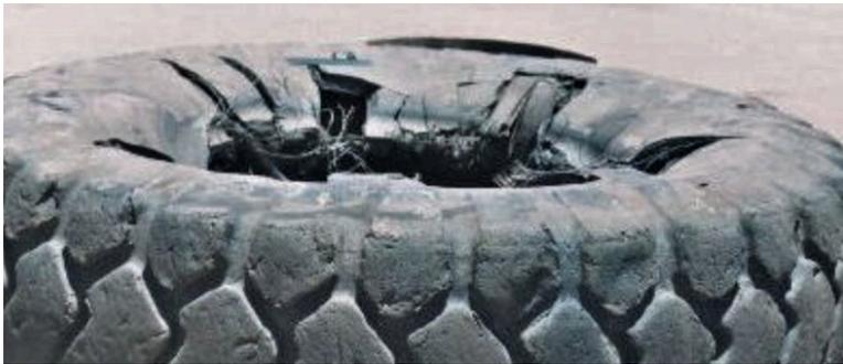
**Figure 27:** Tyre explosion resulting from contact with high voltage line. These can also lead to tyre fires.
