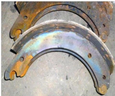
**Figure 20:** Trailer drum brake shoes showing destruction of linings due to dragging brakes
