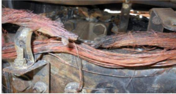
**Figure 12:** A cable rub at a clamp point caused this short-circuit.
