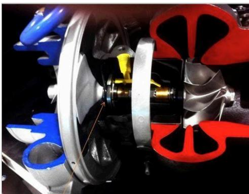
Figure 18: The turbocharger oil seals shown in a cut-away turbocharger.
