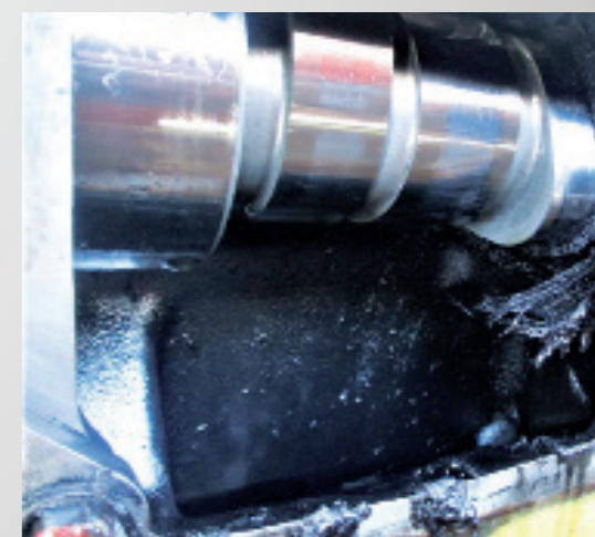
Does the mechanic know how many rags and tools were used on the job? A rag left inside this engine blocked the oil galleries and caused crank and cam bearing failure.
