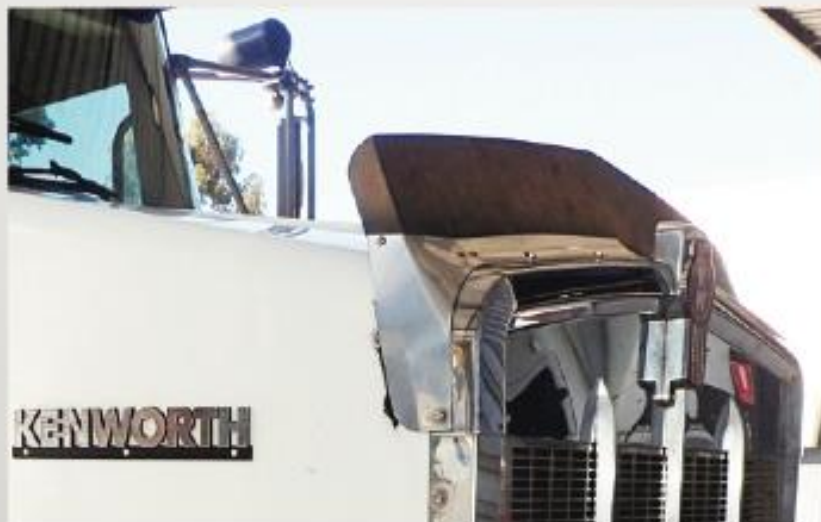
Figure 1: An opaque bug deflector on a bonnet truck is probably illegal.
