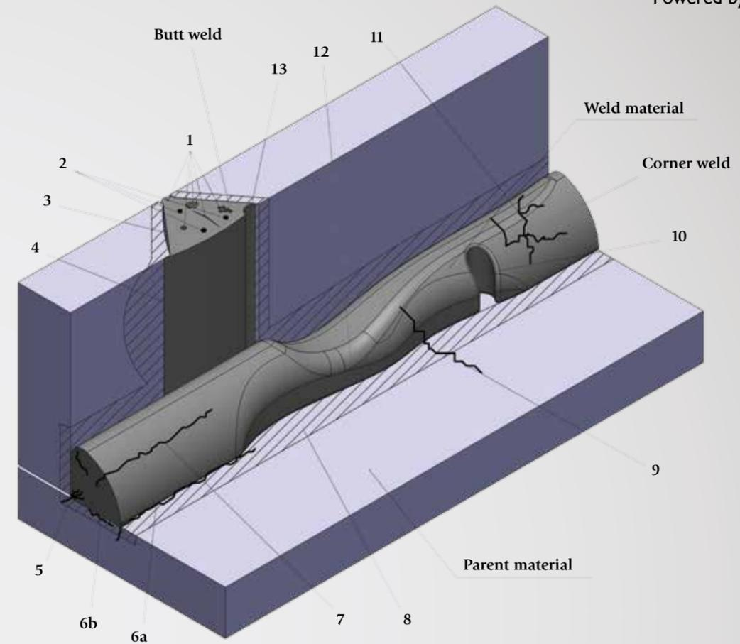
**1. Fine/coarse cluster porosity/blow holes and hollow root beads:**
