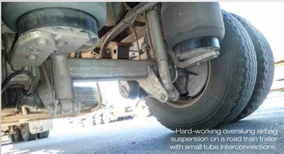
Hard-working overslung airbag suspension on a road train trailer with small tube interconnections.
