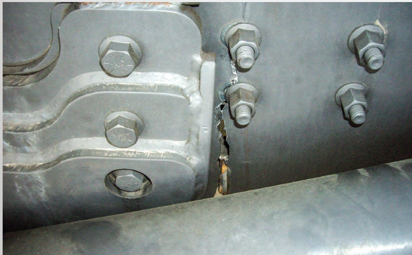
Image 1: Chassis rail cracking near to a lifting cylinder attachment mid-chassis on a tilting compactor
