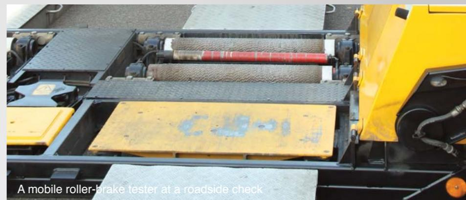
A mobile roller-brake tester at a roadside check
