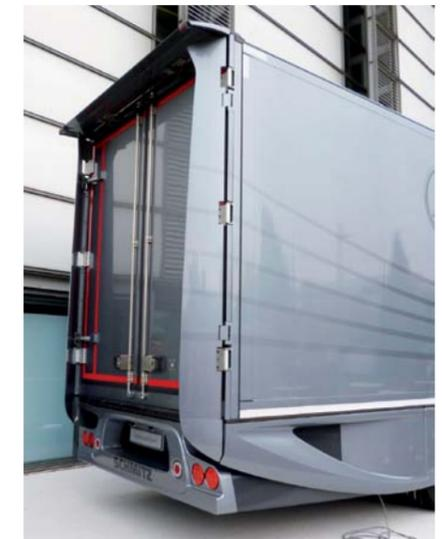
**"The total aerodynamic styling package is claimed to reduce the fuel consumption by 4.5 per cent."**
