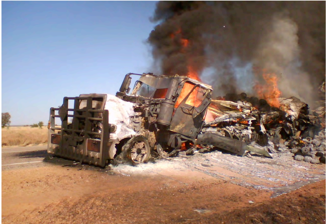
A distressing sight. Loss of a road train prime mover due to an engine compartment fire.
