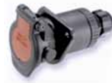
ISO 7638-1 (24V) or ISO 7638-2 (12V) seven-pin EBS braking connector. Power, return and CAN bus for electronic braking systems.
