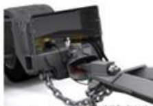
Example of safety chains fitted between the trailer drawbar and truck towbar. Source: Bartlett Equipment
