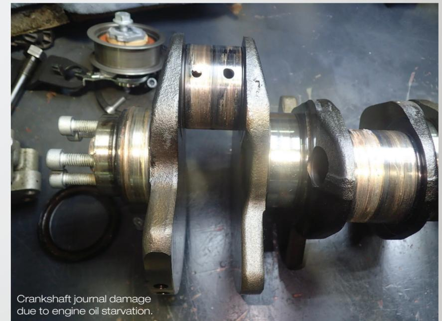
Crankshaft journal damage due to engine oil starvation.
