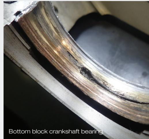
Bottom block crankshaft bearing.
