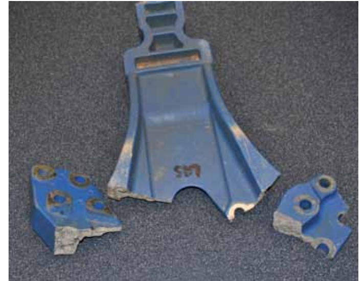
This non-genuine cast aluminium suspension pedestal has failed because of casting porosity. Parts that could cause a crash if they fail should always be genuine or certified acceptable.
